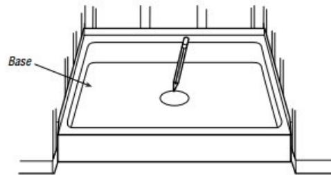
1.3 Cut drain access and install drain pipe.
