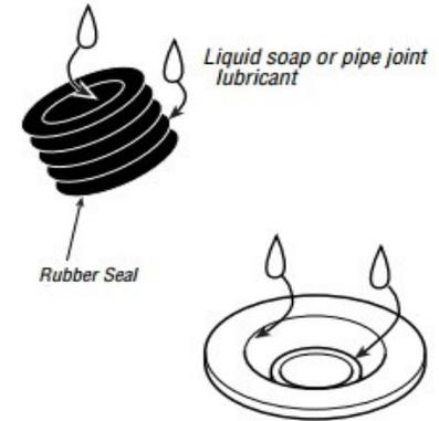
2.3 Insert rubber seal and tap down until flush with drain pipe.
